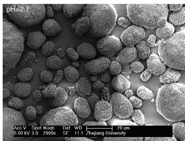
Figure 9 SEM images of the resulting particles at various pH value with \tau = 47 min.
